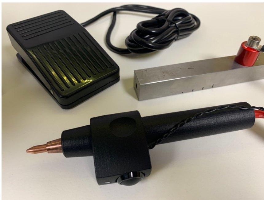
Figure 3. The SPW-1 welding-head and trigger switches
