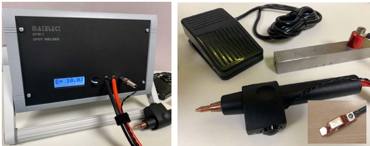
Figure 17. Key component parts of the Matelect SPW-1 universal spot-welder. LHS – main unit, with welding head attached. RHS – foot-switch, magnetic clamp and (inset) alternative sprung copper clamp.
