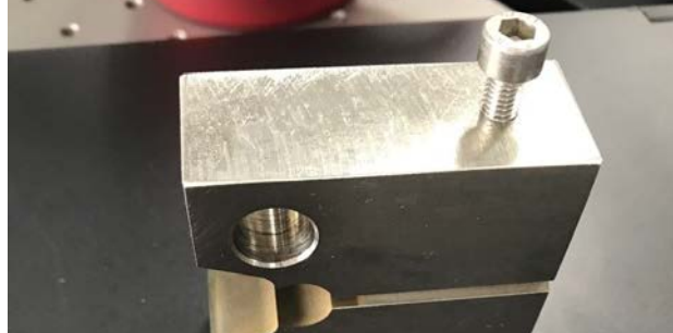
Figure 3 Screwed current connections (DCPD) into a CT specimen
