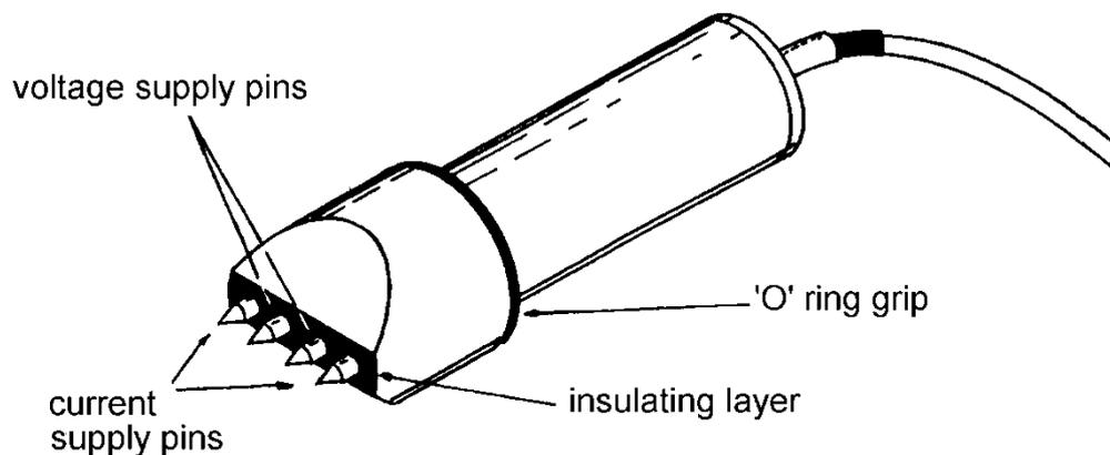
*Figure 1 - Basic configuration of the Matprobe-2*
