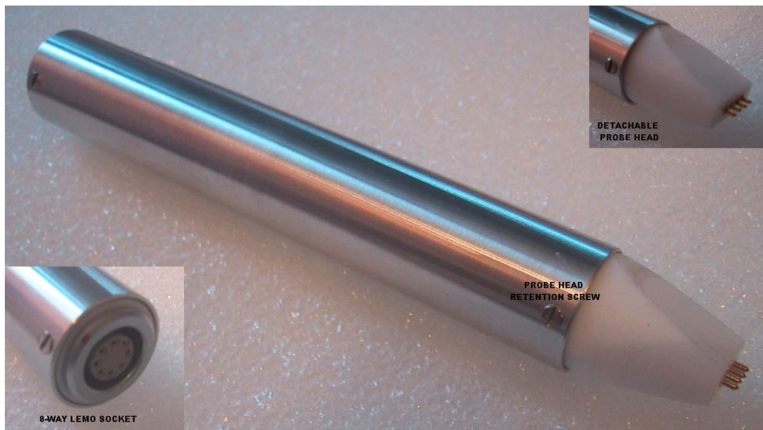
Figure 1 - Basic configuration of the Matprobe-2
